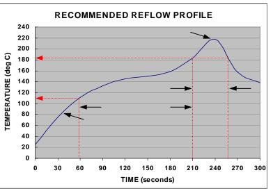
Figure 26. Recommended Reflow profile.
