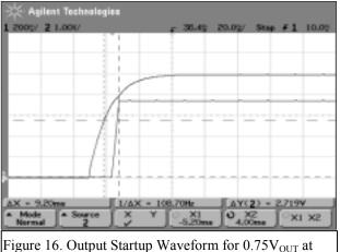
$V_{IN} = 5V$ ,  $I_{OUT} = 18A$ .
