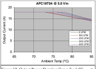
Figure 12. Output Power Derating Curve for  $1.5V_{OUT}$  at  $V_{IN} = 5V$ ,  $T_A = 25^{\circ}C$
