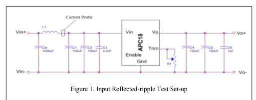
Measure input reflected current with a simulated source inductance L1 of 1uH. Capacitor Cin offsets possible battery impedance. Measure current as shown above.
